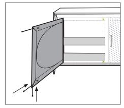
7 Insert two poles horizontal and one pole vertical. The thin pole must be curved and attached at top and bottom pocket
